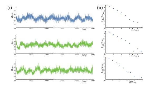
Figure 5: Plots of the sticking codimension  $n_{stick}$  for systems of 200 oscillators for three different sets of spring and damping coefficients in (i), and the frequency of stick-slip cascades of size  $\Delta n_{stick}$  in (ii) shows a logarithmic pattern for each system in (i).
