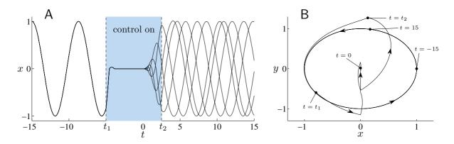
Figure 9: Panel A shows five sample solutions to (5.2) using (5.5), (5.6) and  $\varepsilon = 0.001$ , and the initial condition (x, y) = (1, 0) at t = -15. The control (5.3) causes the solutions to pass close to a two-fold at t = 0, effectively randomising the phase. Panel B shows one of the solutions in phase space, with the location of the solution highlighted at key times. The sample solutions were computed using the Euler-Maruyama method with a step-size of  $\Delta t = 10^{-5}$ .
