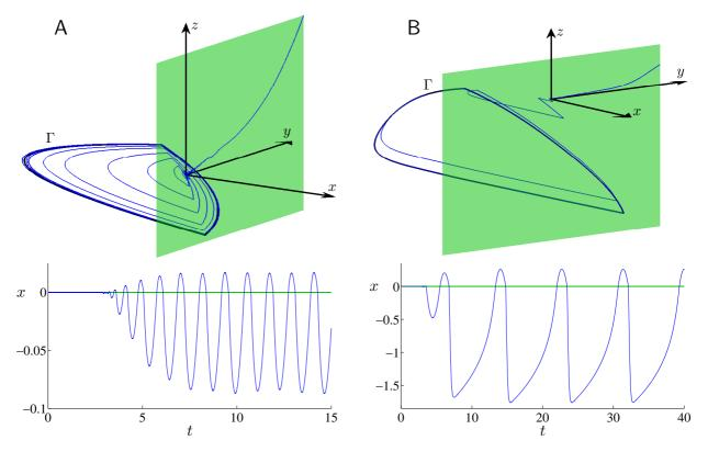
Figure 7: Panel A shows a typical sample solution, both in phase space and as a time series, for (4.1) with (3.5) and (3.6) using D = I and  $\varepsilon = 0.001$ . Panel B shows an typical sample solution using instead (4.2). Both solutions start at X = (0, 1, 1), pass near the two-fold X = (0, 0, 0), then approach a stable periodic orbit  $\Gamma$ . The solutions were computed using the Euler-Maruyama method with a step-size of  $\Delta t = 10^{-5}$ .
