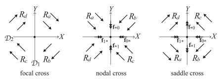
Figure 8: Three sliding geometries that form focus-like, node-like, and saddle-like, equilibria in the X-Y subsystem. The assignment of the regions  $R_{a,b,c,d}$  are shown. The sliding vector fields  $\mathbf{f}_{\star i}$  on  $\mathcal{D}_1$  and  $\mathbf{f}_{i\star}$  on  $\mathcal{D}_2$  are labeled.
