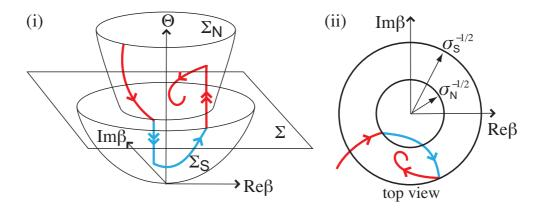
FIG. 6: (Color online) Example of an orbit of the Filippov system. (i) In the 3-dimensional phase space  $(\text{Re}\beta, \text{Im}\beta, \Theta)$ , orbits are attracted to and slide on the switching manifolds  $\Sigma_N$  and  $\Sigma_S$ , (ii) projection onto the complex  $\beta$  phase plane, showing intersections of the switching manifolds  $\Sigma_{N,S}$  with the switching manifold  $\Sigma$ . Fast dynamics are shown with double arrows, sliding orbits with single arrows.
