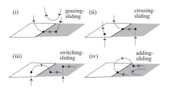
FIG. 1: Phase portraits for the four sliding bifurcations in three dimensions. The discontinuity manifold is represented by a horizontal plane in which the attracting sliding region is shaded.
